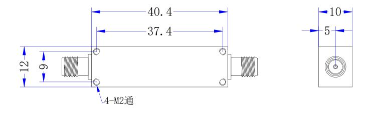
Units: mm/[inch], Tolerance: ±0.5mm, Mounting Hole Tolerance: ±0.2mm
