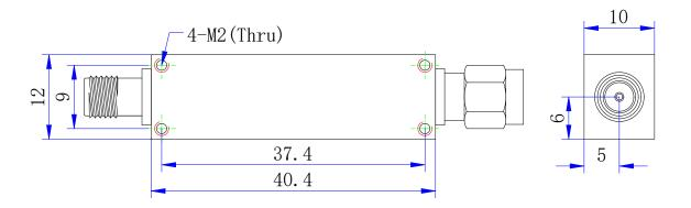
Units: mm/[inch], Tolerance: ±0.5mm, Mounting Hole Tolerance: ±0.2mm Note 1: Excluding Connectors
